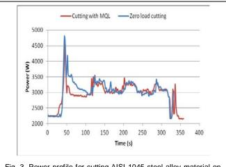
Fig. 3. Power profile for cutting AISI 1045 steel alloy material on the Roeders RFM 760 high speed milling machine.
